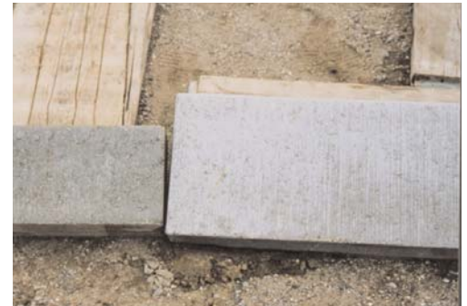
IS blended cement (33 percent slag content) was used to produce a noticeably lighter concrete masonry unit on the right.
